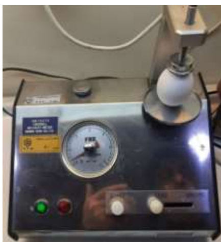
Fig 1. Eggshell Strength Measurement Device
