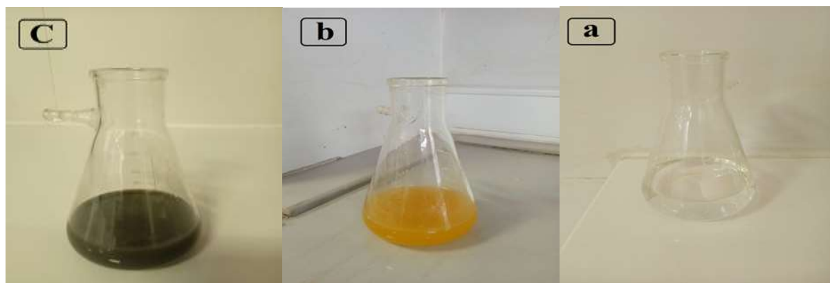
Figure (1) Color change of aqueous extract of dried tomato pomace after adding silver nitrate (a) colorless silver nitrate solution (b) Aqueous extract of dry tomato pomace (orange color) (c) Formation of silver nitrate colloidal dispersion and aqueous extract whose dark color indicates the formation of silver nanoparticles after pH adjustment
