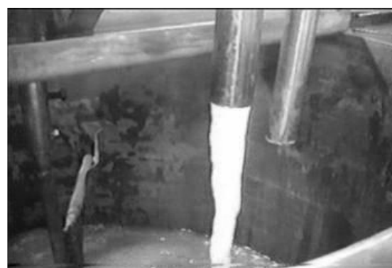
Figure 3 Water phase receive in emulsion tank
