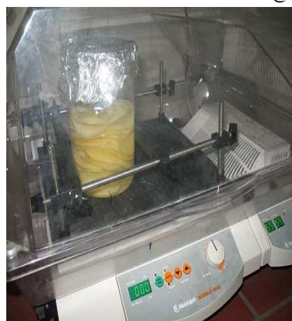
Fig 2 Starch extraction from potato slabs in shaker-incubator
