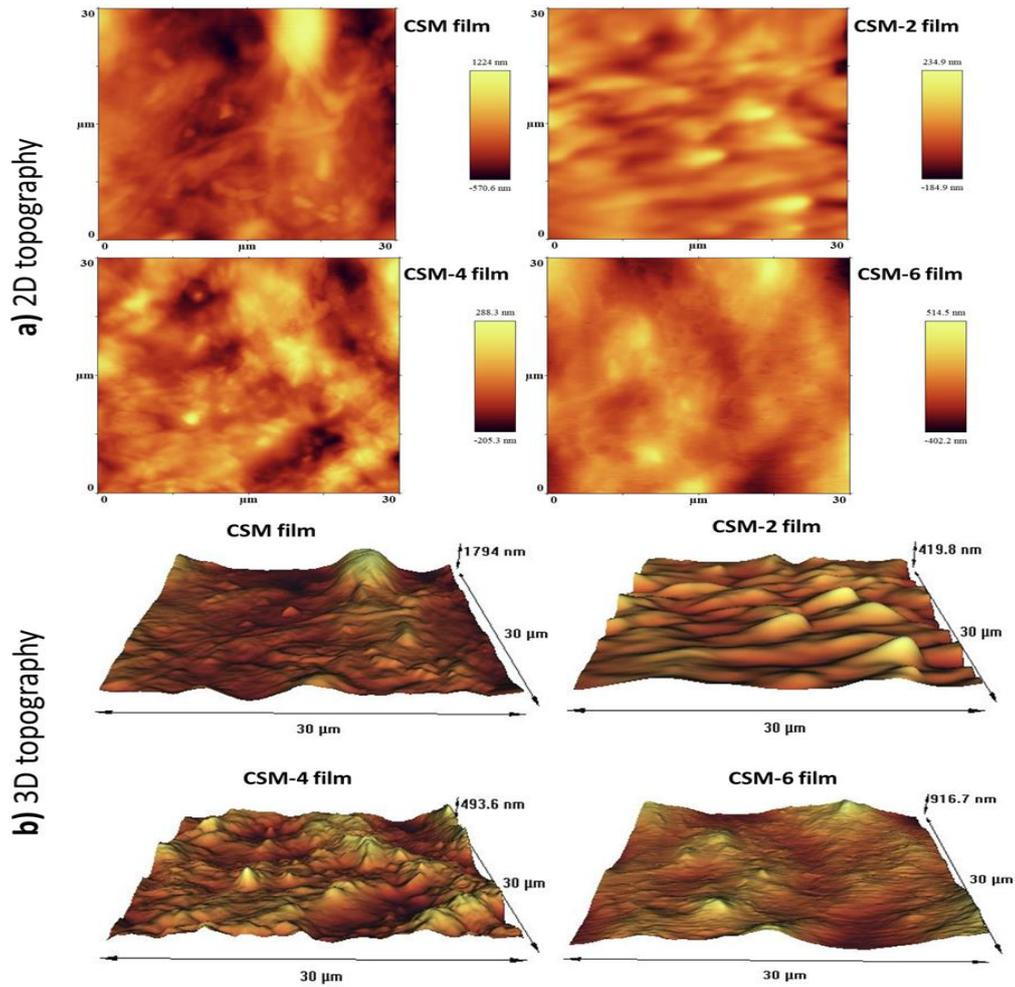
**Fig. 2.** AFM images of 2D surface (a) and 3D topography (b) of chia seed mucilage (CSM) films with different concentrations (2, 4, and 6%) of cinnamon essential oil nanoemulsion.
