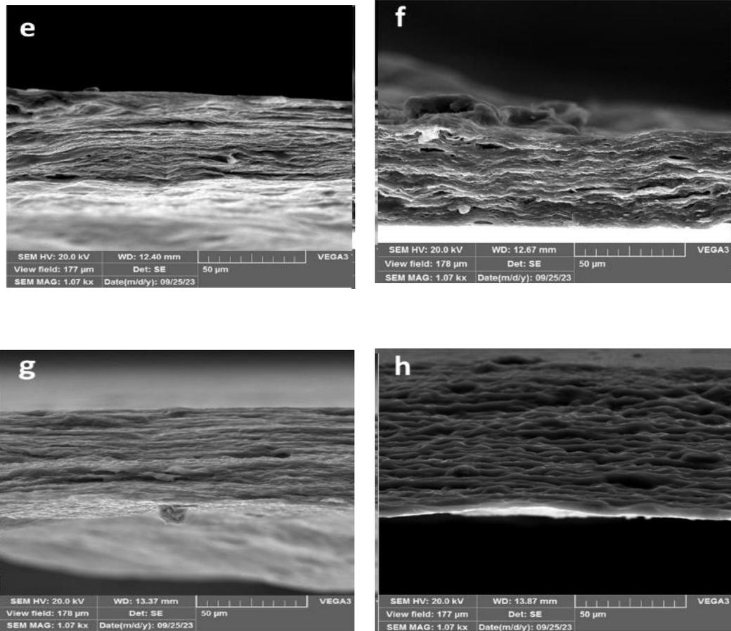
**Fig. 1.** SEM images of the cross-section of CSM film (e), CSM-2 (f), CSM-4 (g), CSM-6 (h).
