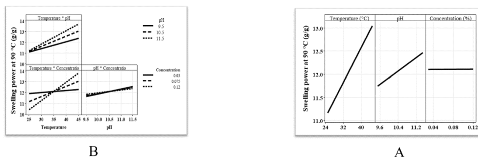
Fig 5. Simple and reciprocal effects of temperature, pH and reactant concentration on swelling power of phosphorylated wheat starch at 90°C.
