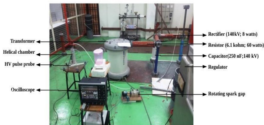
Figure 4: The pulse electric circuit experimental setup
