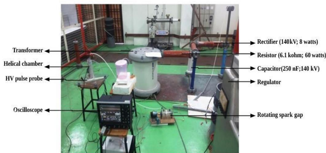
Figure 4: The pulse electric circuit experimental setup
