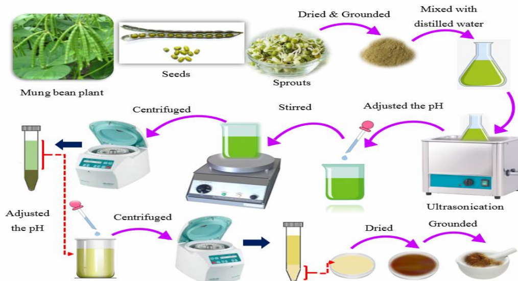
Fig 1 Schematic diagram of production of SMPI by ultrasonic pretreatment/alkaline extraction and acid precipitation.
