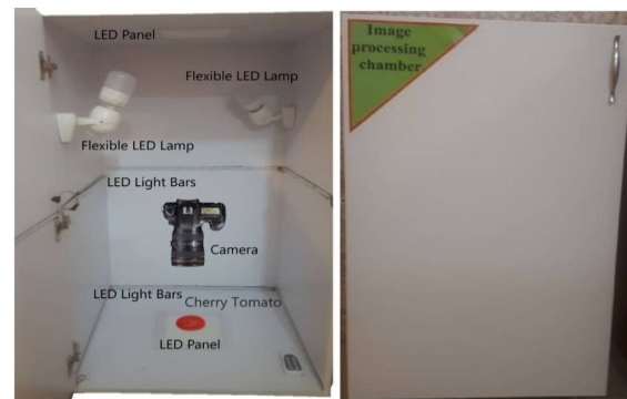
Fig 1 Scheme of Artificial vision system (AVS) set-up.
