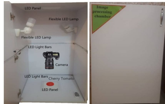
Fig 1 Scheme of Artificial vision system (AVS) set-up.
