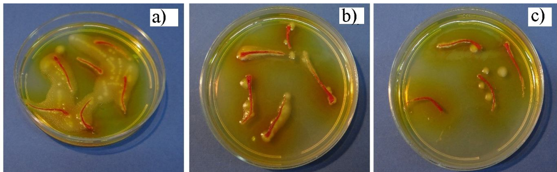
Fig 6 Bacterial disinfection effects of dielectric barrier discharge plasma in surface mode for a) control and b) 15 second c) 15 second plasma treated sample
