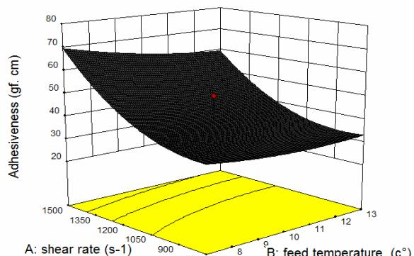
**Fig 2** Effect of extruder shear rate and feed temperature on adhesiveness of butter (storage temperature of  $10^{\circ}\text{C}$ )
