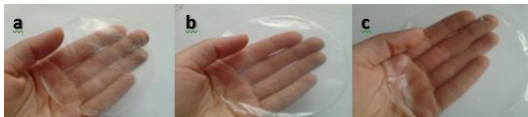
Fig 1 Illustrative picture of films made from (a) Alyssum homolocarpum seed gum, (b) tragacanth gum and (c) locust bean gum
