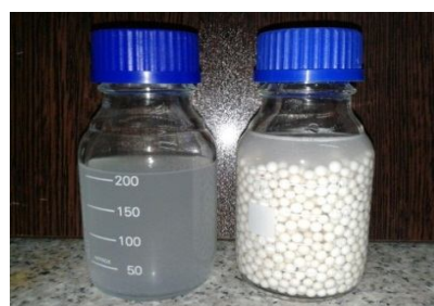
Fig 1 Yeast cell suspension (In the left image) and Alumina silicate with cell suspension (in the right)
