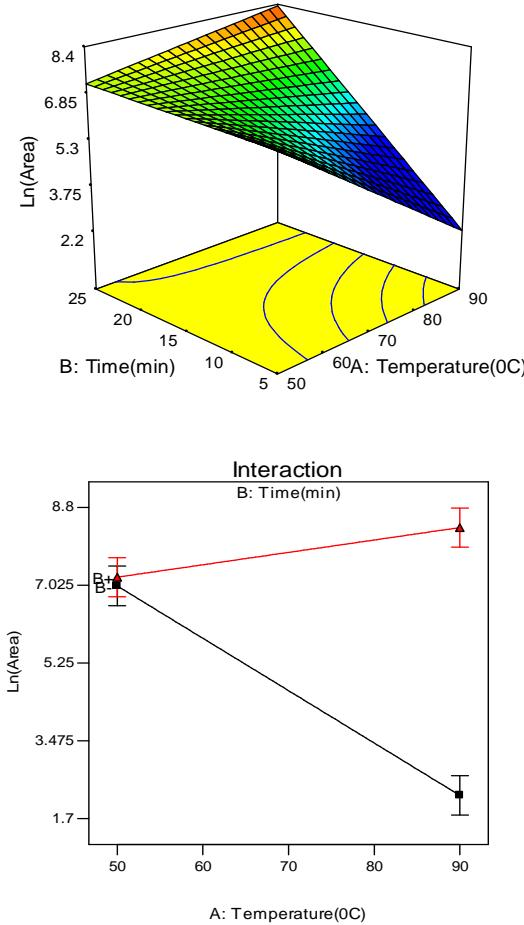
**Fig 2** Response surfaces of total peak area based on temperature and time of extraction
