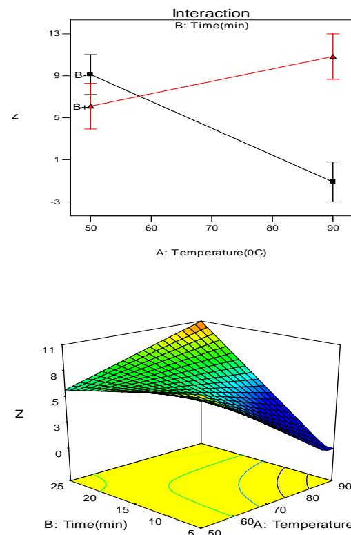
**Fig 1** Response surfaces of total peak number based on temperature and time of extraction
