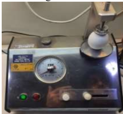
Fig 1. Eggshell Strength Measurement Device
