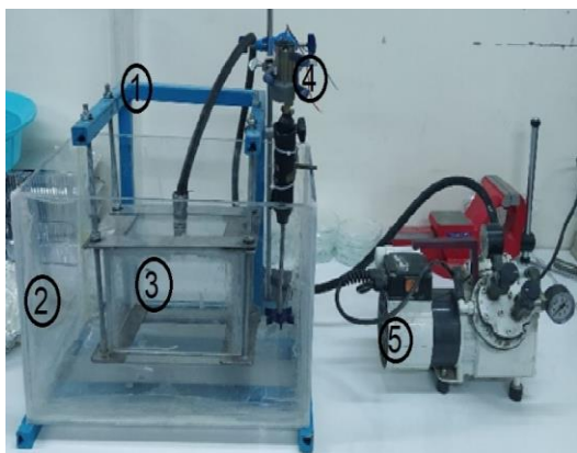
Figure 5: Vacuum-built filter system
