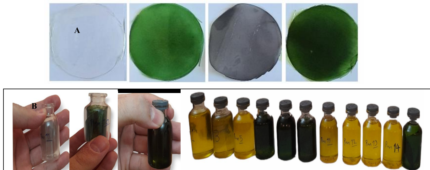
Fig 1 Examples of prepared films (A) and packaging of virgin olive oil with prepared films (B)
