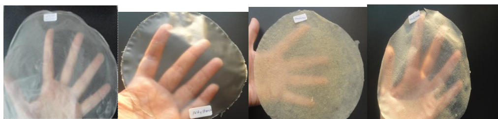
Fig 2 Composite films of starch-Olibanum, starch-Zein, starch-PVA and control (starch), from right to left respectively.
