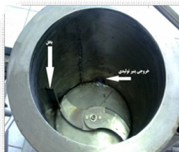
F 1 Developed cooking machine for processed cheese
