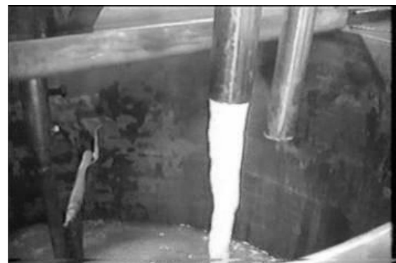
Figure 3 Water phase receive in emulsion tank
