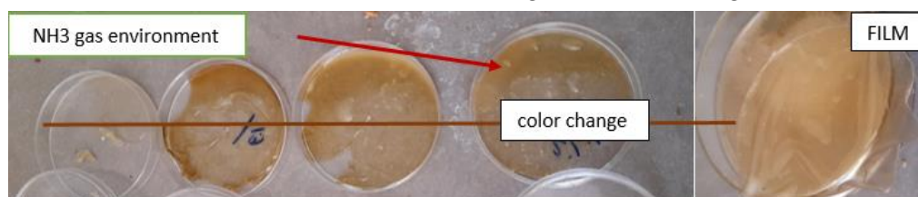
Figure 4. Changes of biogenic gases on the film containing anthocyanin marker extracted from basil stem ( Ocimum basilicum )
