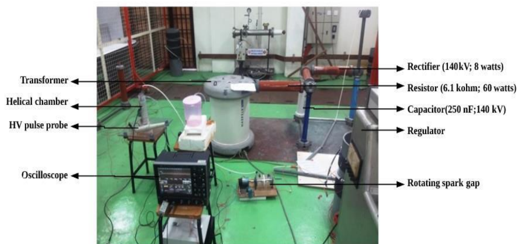
Figure 4: The pulse electric circuit experimental setup
