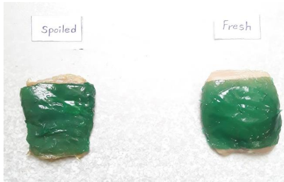
Fig 5) Color changes in the intelligent pH indicator PS-films on the chicken fillets after 0 and 8 days of storage at 4 °C for fresh and spoiled chicken, respectively.
