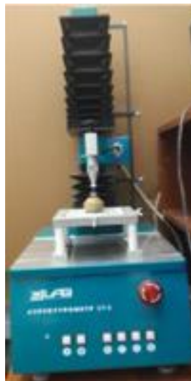
Figure 1 Appearance of the ST-2 Structurometer
