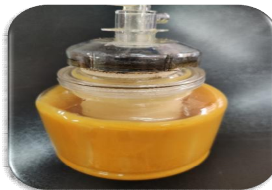
Fig 3 Dissolved solid particles (pulp) stuck to the wall of the separator vessel used
