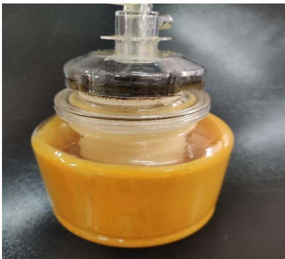
Fig 2 Semi-continuous separator rotary separator vessel 1: fluid inlet containing pectin 2: fluid outlet 3: separated solid part stuck to the wall of the vessel due to rotational force (undesired part) 4: separated dilute fluid part leaving (desirable part)
