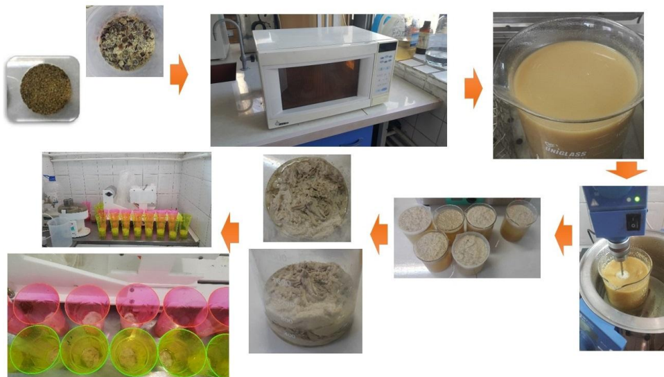
Fig 1 Microwave-assisted extraction of galactomannans from plant seeds
