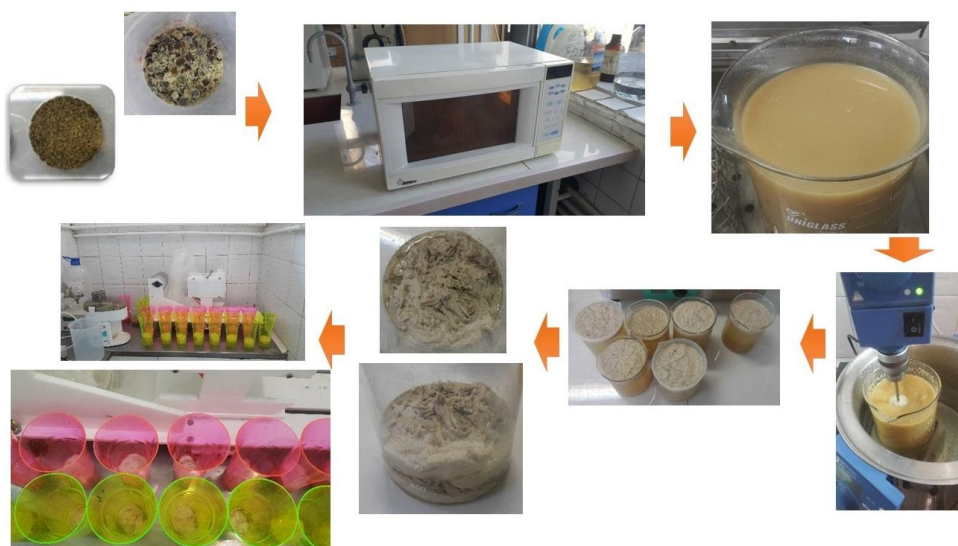
Fig 1 Microwave-assisted extraction of galactomannans from plant seeds
