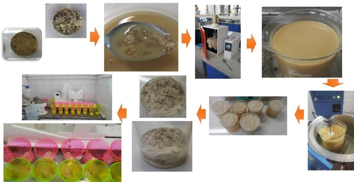
Fig 1 Ultrasound-assisted extraction of galactomannans from plant seeds
