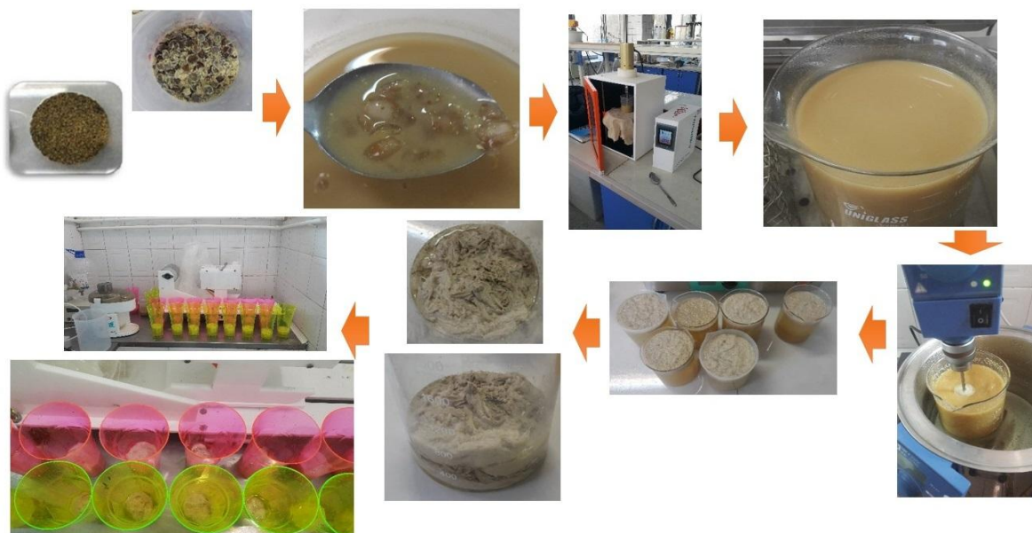
Fig 1 Ultrasound-assisted extraction of galactomannans from plant seeds
