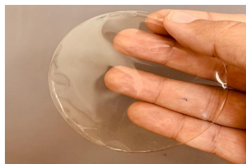
Fig 9 Optimized edible film based on gelatin-Persian gum
