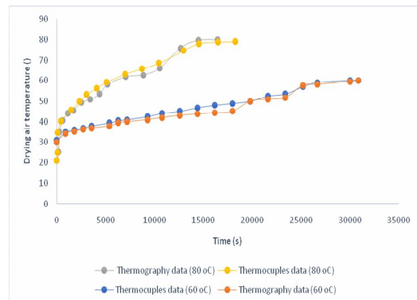
Fig 5. Evaluation the temperature change by infrared thermography and thermocouple in different drying air temperature (60 and 80 °C)
