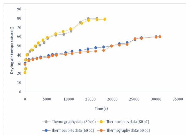
Fig 5. Evaluation the temperature change by infrared thermography and thermocouple in different drying air temperature (60 and 80 °C)
