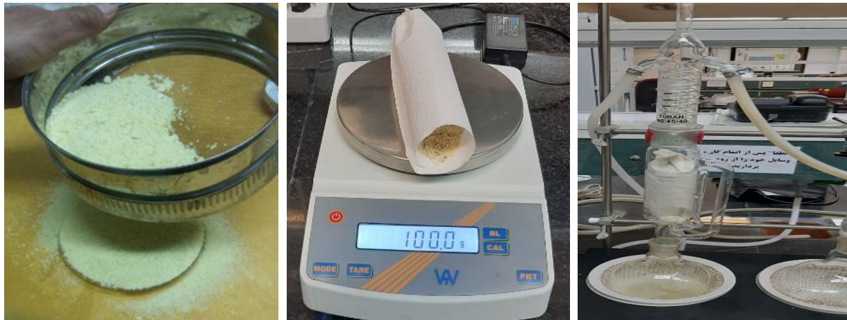
Fig 3 Steps of sample preparation for placement in Soxhlet set.
