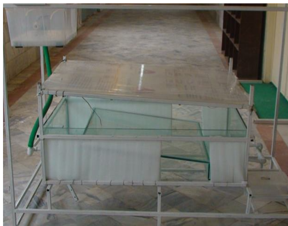
Fig 2 Photograph of the continuous UV-C irradiation system.
