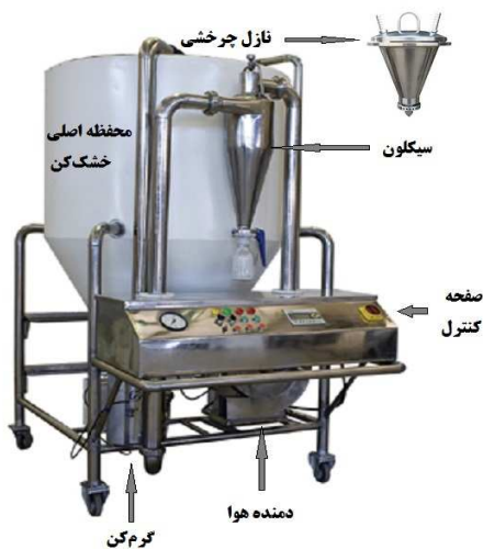
Fig 1 pilot scale spray dryer used in this study.
