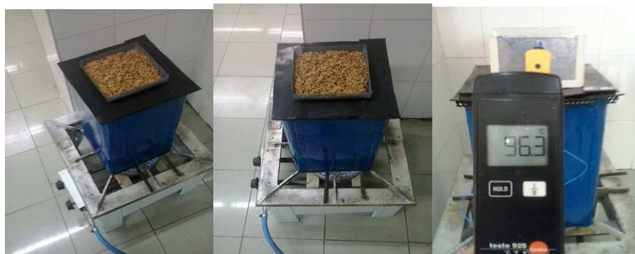
Fig 2 System of paddy steaming with showing of steaming temperature
