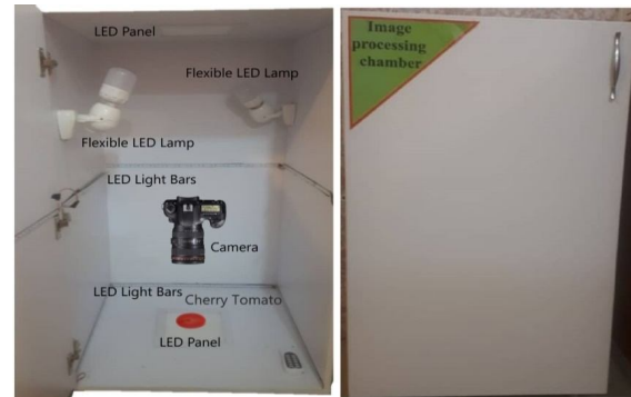
Fig 1 Scheme of Artificial vision system (AVS) set-up.
