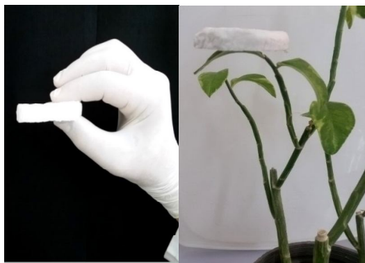
Fig 5 Production of cellulose nanofibers aerogel from date palm.
