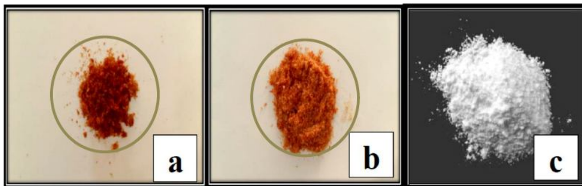
Fig 1 pure pomegranate peel extract powder (a) inclusion complex of \beta -CD and pure pomegranate peel extract powder (b) \beta -CD powder (c)
