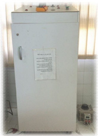
Fig 2 Pulsed electric field system- Research Institute of Food Science and Technology
