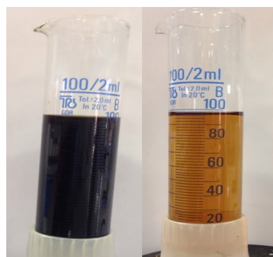
Fig 5 The image of clarified molasses syrup (right side) was refined at optimum condition and its comparison with control sample (left side).
