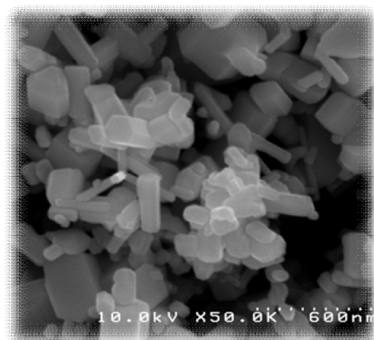
Fig 1 ESEM image of nanoparticles of zinc oxide.
