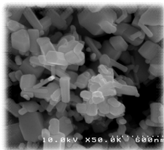
Fig 1 ESEM image of nanoparticles of zinc oxide.
