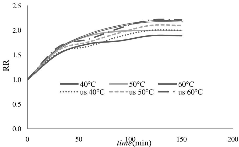
**Fig 4** Rehydration rate curves of dried Poulk (*Stachys Sctachgeleevii Sosn.*) untreated and submitted to ultrasonic treatment (us) at 1m/s and temperature of 40, 50 and 60°C.
