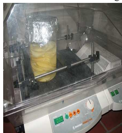
Fig 2 Starch extraction from potato slabs in shaker-incubator
