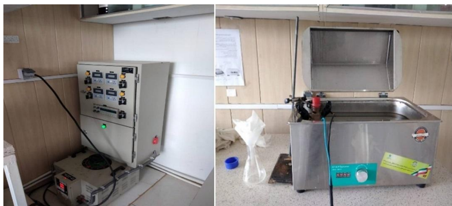
Fig 1 Ohmic heating system.
