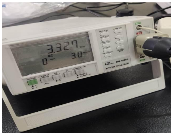
Fig 5 A view of the used Lutron DW-6090A power analyzer
