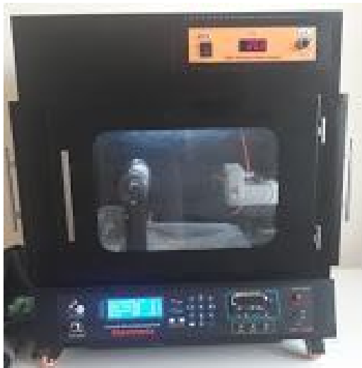
Fig 1 Electrospinning device used in this study
